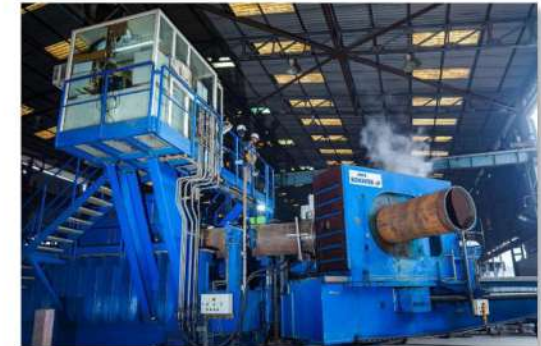
Induction bending process
