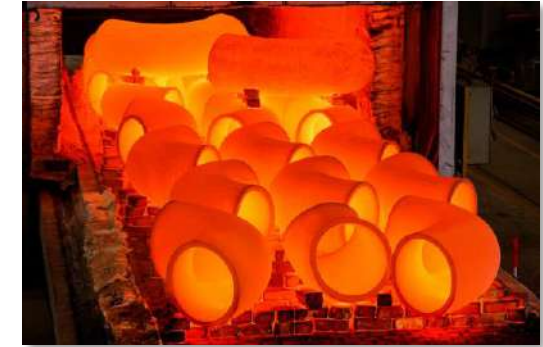
Fully CNC heat treatment furnaces (gas and electric)
