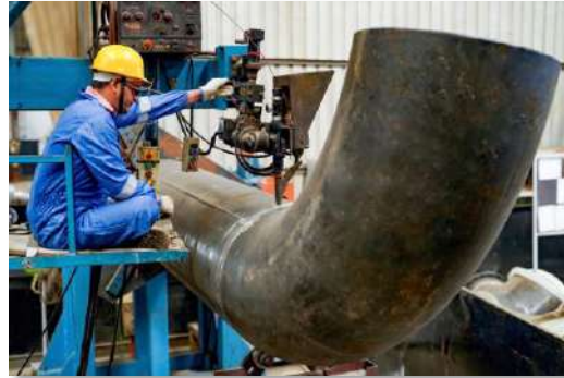
Automatic GMAW Welding System
