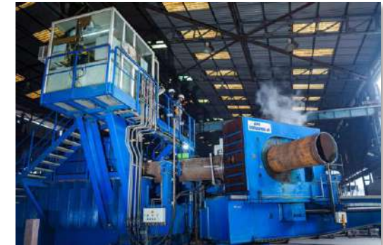
Induction bending process
